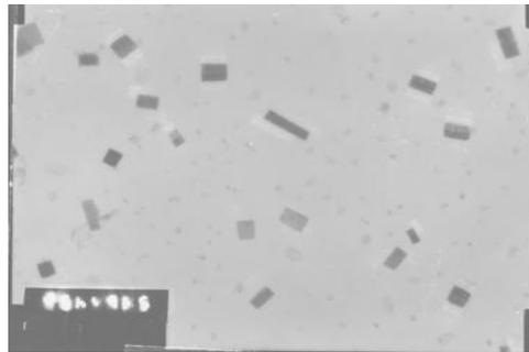
Fig. 7 : TEM image showing formation of ZnO due to ageing
