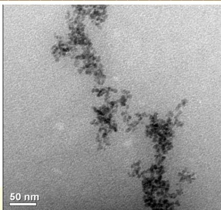
Fig. 2 (b) : HRTEM image of ZnS nano particles
