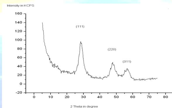
Fig. 1 (a) : X-ray diffractogram of ZnS
