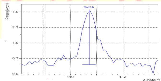
Fig. 6(b) : XRF spectra of S of ZnS
