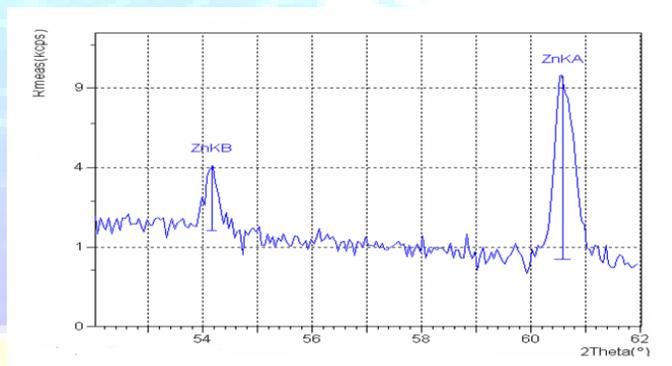
Fig. 6 (a) : XRF spectra of Zn of ZnS
