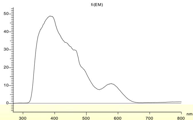
Fig.5 : PL spectra of ZnS doped with Mn
